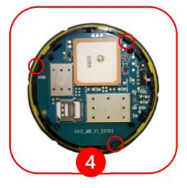
Locate three small clips holding unit in place.
