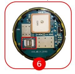
Locate the SIM tray on the top of the device.
