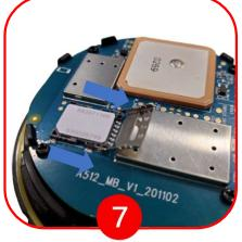
Slide tray cover to unlock, open and insert the new SIM card with the gold contacts facing down.
