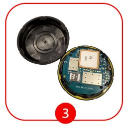
Once unlocked, pull cover off the device.
