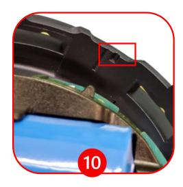
Component should align with grooves on side of case, push in until all three clips (step 5) make a clicking sound.
