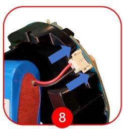
Connect new battery and put into device.
