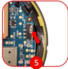
Locate the power switch on the side of the device and slide it to the "ON" position.
