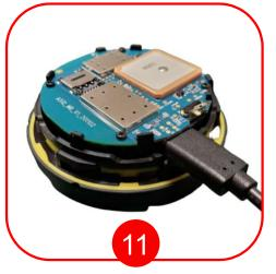
Plug device into a computer using the USB C port and send battery replacement command (AT+GTRTO) via Micron MAP Utility program. Reset device after command acknowledged.
