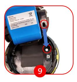
Align sensor hole on case with sensor hole next to battery, push component back into place.
