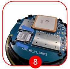
Close and lock the SIM card tray by sliding it forward, then turn on the device after installing new SIM card.
