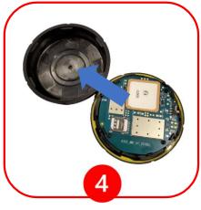
Once unlocked, pull cover off device.
