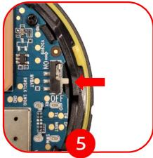
Locate the power switch on the side of the device and slide it to the "OFF" position.
