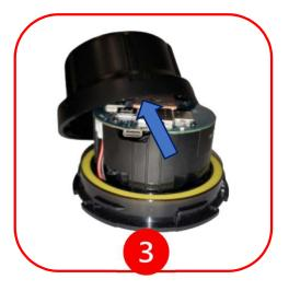
Once unlocked, pull cover off the device.
