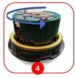
Twist counterclockwise to unlock center component from base.
