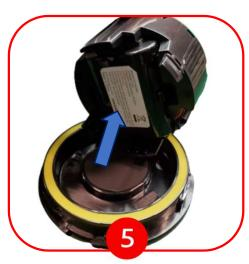
Once unlocked, pull component out of the case.
