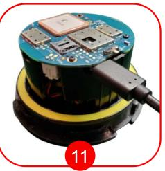
Plug device into a computer using the USB C port and send battery replacement command (AT+GTRTO) via Micron MAP Utility program. Reset device after command acknowledged.
