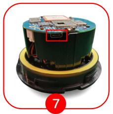
Use the USB C port located on the side of the device (under the ON/OFF switch) for programming device commands.
