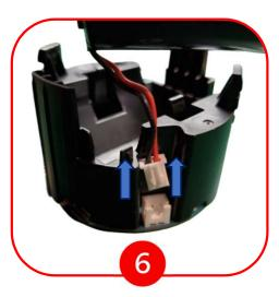
With the battery facing up, pull out old battery and unplug from device.
