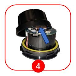
Once unlocked, pull cover off device.
