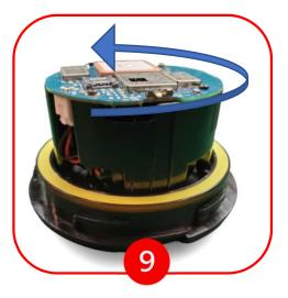
Twist device clockwise, interlocking teeth on base with threading on component, until it makes a clicking sound.
