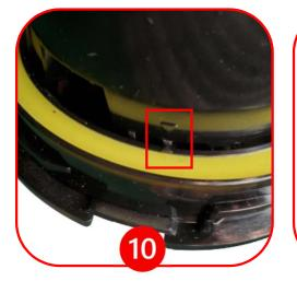
Ensure the embossed guide arrow on side of device lines up with corresponding arrow on rim of the base.
