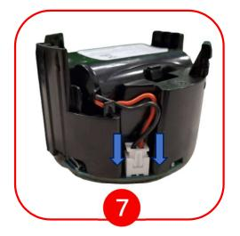
Connect new battery and put into device.
