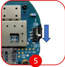
Locate the power switch on the side of the device and slide it to the "OFF" position.
